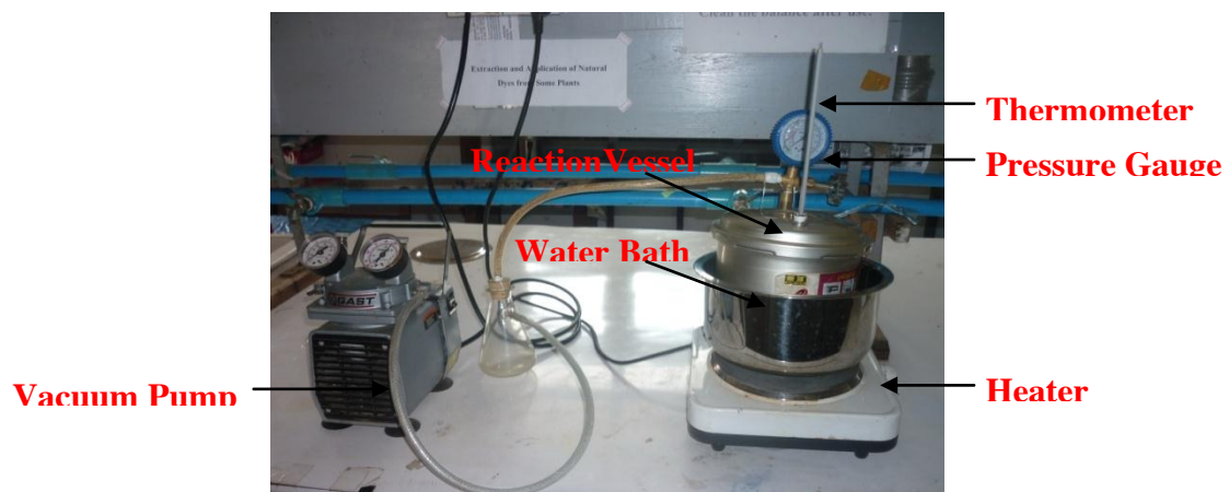
Figure (1) Makeshift Vacuum Evaporator
